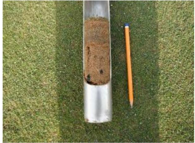
Figure 2: 3mm of unchecked organic matter had accumulated at the top of the profile on the 12<sup>th</sup> green which was typical of all. The mild weather over the last few months had contributed while no sand was purposely applied to avoid heightening the disease pressure after last year's outbreak.
